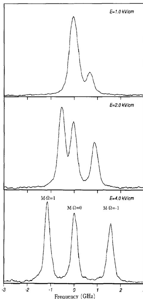
Fig. 2. Observed splitting of the  $R_2(0)$  transition of CO around  $48478.48 \text{ cm}^{-1}$  as a function of the electric field in the excitation region. The polarization vector of the excitation laser is chosen such that all  $\Delta M$  transitions appear equally strong. Due to the fact that  $M=0$  states with different parity do not interact, only the transition to the  $M=0$  state with parity is observed.
