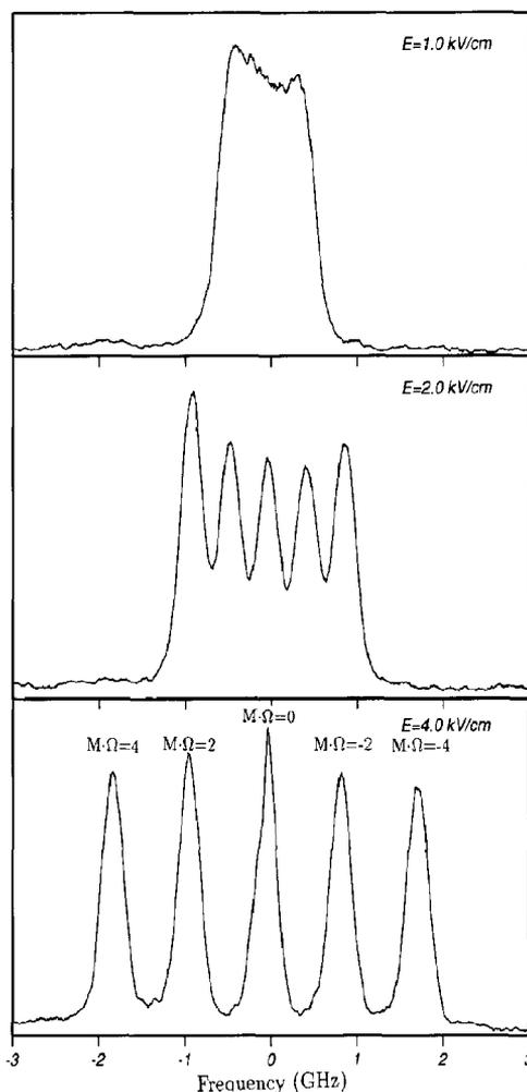
Fig. 3. Observed  $R_3(1)$  transition of CO as a function of the electric field in the excitation region, again with an angle between the polarization vector of the laser and the applied electric field close to the magic angle of  $54.7^\circ$ .
