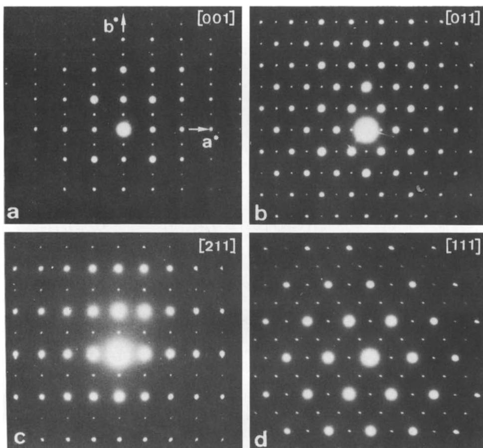
Fig. 7. Electron diffraction patterns of the simple cubic low-temperature phase. (a) [001] zone; note the presence of the  $0k0$  row with  $k = \text{odd}$  due to double diffraction. All reflections with  $h = \text{odd}$  are systematically absent. (b) [011] zone. (c) [211] zone. (d) [111] zone.
