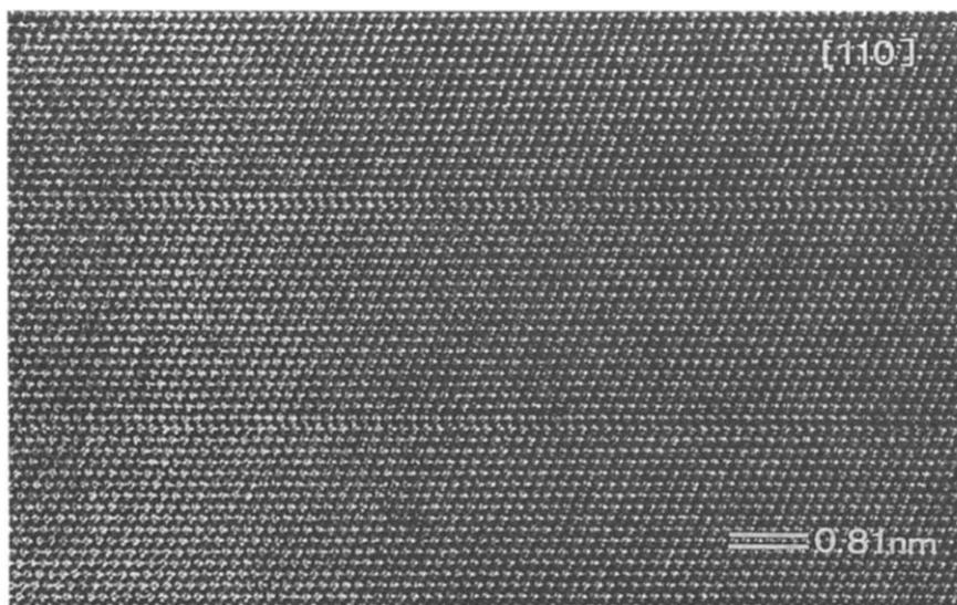
Fig. 5. Stacking faults in pure  $C_{60}$  imaged along  $[110]$ .
