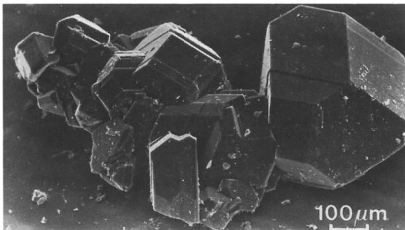
Fig. 1. Scanning electron micrograph of single crystals of  $C_{60}$  obtained by vapour transport.
