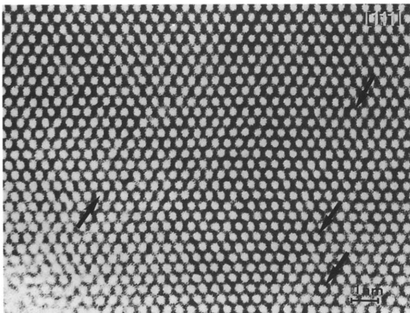
Fig. 4. High-resolution image of  $C_{60}$  crystal containing 10% of  $C_{70}$  viewed along the [111] zone. Note the local differences in dot brightness attributed to the presence of  $C_{70}$  molecules.
