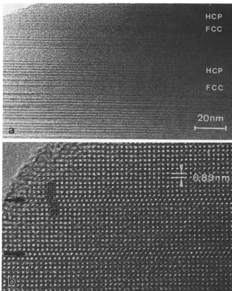
Fig. 13. (a) Low-magnification high-resolution image along  $[2\bar{1}10]_{\text{HCP}}$  or  $[110]_{\text{FCC}}$  showing the interweaving of FCC and the HCP bands. (b) High-resolution image of a HCP stacked region; two stacking faults are indicated by arrows.
