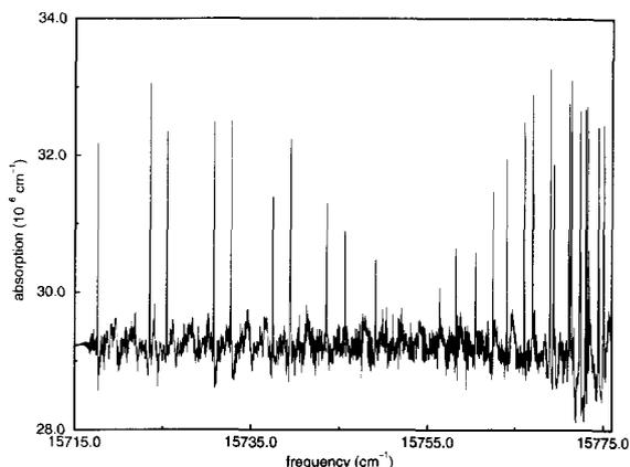
Fig. 2. The absorption spectrum of 365 mbar of  $^{18}\text{O}_2$  around 635 nm measured via the PS-CRD method. The spectral structure is due to the  $b^1\Sigma_g^+(v' = 2) \leftarrow X^3\Sigma_g^-(v'' = 0)$  transition.
