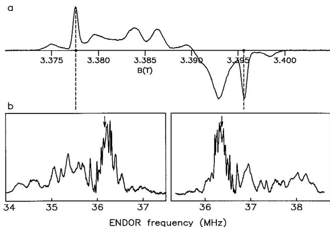
**FIG. 2.** ESE-detected EPR (a) and  $^{13}\text{C}$ -pulsed ENDOR (b) spectra at 95 GHz and 1.2 K of a single crystal of  $^{13}\text{C}_{60}$  for the magnetic field parallel to [110]. The ENDOR spectra are taken at fields of resonance of triplet  $\gamma$ . The arrows indicate the  $^{13}\text{C}$  Zeeman frequencies.
