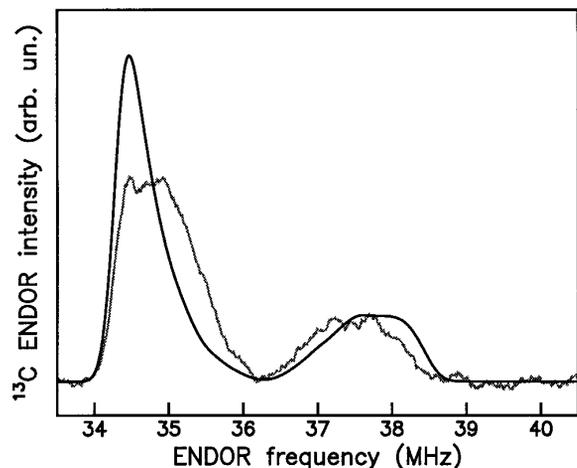
**FIG. 3.** Calculated  $^{13}\text{C}$ -pulsed ENDOR spectrum at a magnetic field of 3.389 T for a hypothetical triplet  $^{13}\text{C}_{60}$  molecule with uniform spin-density distribution. The isotropic hyperfine interaction parameter  $a_{\text{iso}}$  has been taken as  $-30$  MHz (see text). For comparison the experimental spectrum at the same magnetic field (cf. Fig. 1) is reproduced in gray.
