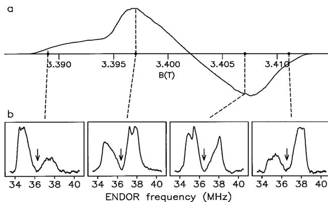
**FIG. 1.** ESE-detected EPR (a) and  $^{13}C$ -pulsed ENDOR (b) spectra of  $^{13}C_{60}$  in decaline/cyclohexane at 95 GHz and 1.2 K. The EPR signal is absorptive at low fields and emissive at high fields. The ENDOR spectra correspond to four different magnetic field settings and the arrows indicate the corresponding  $^{13}C$  Zeeman frequencies.
