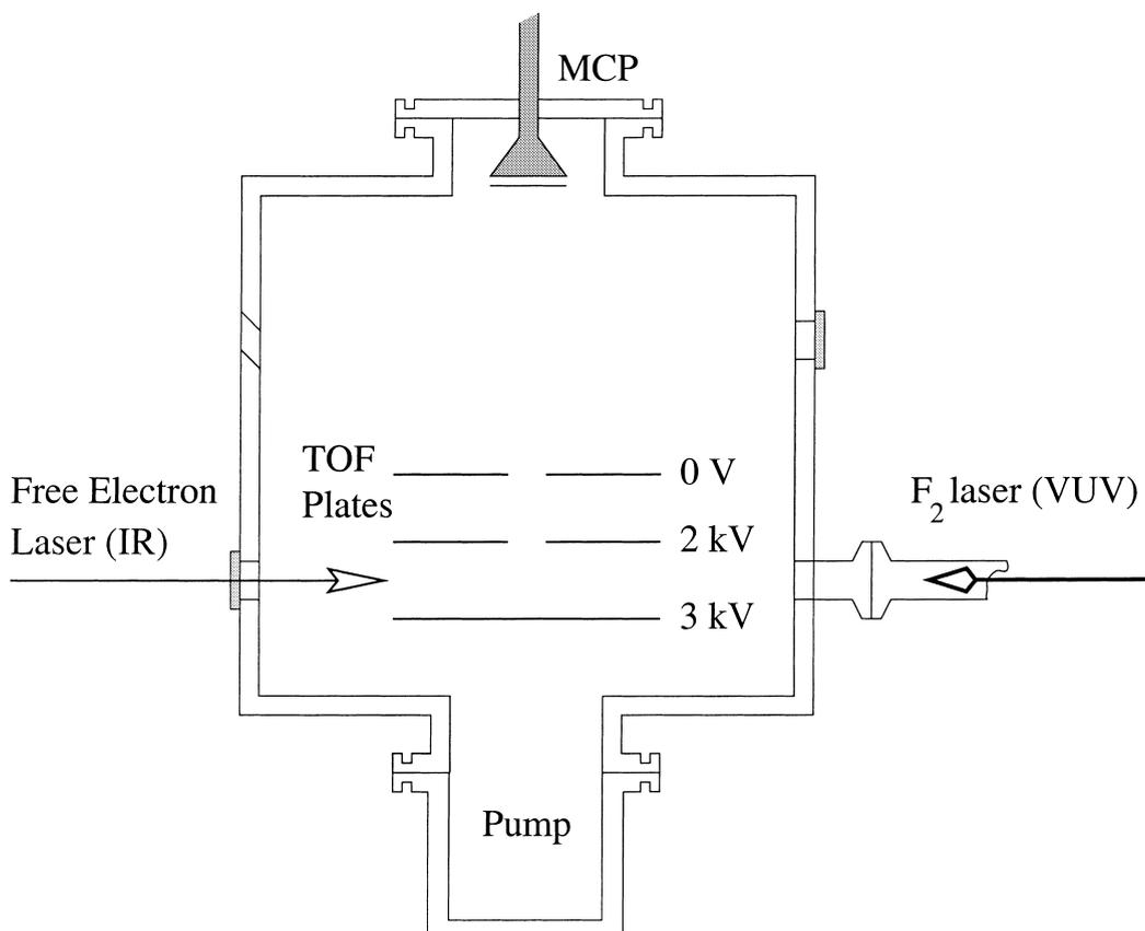
Fig. 1. Schematic of the experimental apparatus. Molecules are ionized between the lower two TOF plates. In the case of the IR/VUV double resonance experiment on PABA, an unfocussed IR and an unfocussed VUV laser are used. In the case of the IR-REMPI experiment on C<sub>60</sub>, only IR light is used which is then focussed by a lens.
