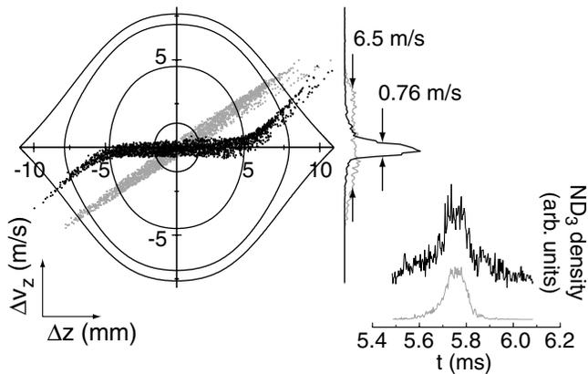
FIG. 4. Calculated longitudinal phase-space distribution at the moment that the buncher is switched on ( $t = 1.743$  ms) and off ( $t = 1.982$  ms) with voltages of  $+3.8$  and  $-3.8$  kV. The projections of the longitudinal velocity distributions on the  $v_z$  axis are given for both cases. On the right hand side, the measured (upper trace) and calculated (lower trace) TOF distributions 33 cm behind the buncher are shown.
