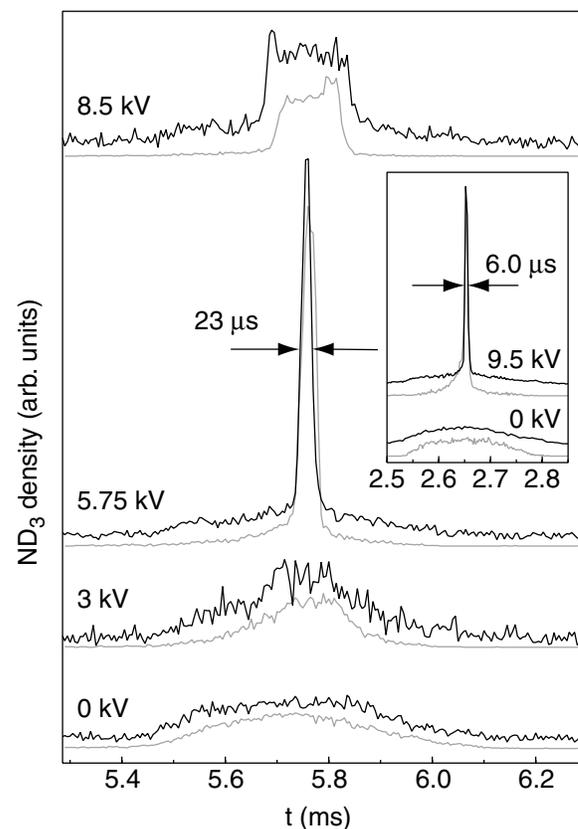
FIG. 3. Density of ammonia molecules 33 cm behind the buncher as a function of time (at  $t = 0$  ms the synchronous molecule is at the exit of the decelerator) for different voltages on the buncher, using two bunching stages. In the inset similar measurements recorded at a 4.5 cm distance behind the buncher, using three bunching stages, are shown. The results of trajectory calculations through the entire setup are shown underneath the experimental data.
