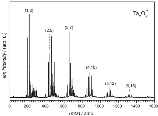
**Fig. 1.** Mass spectrum of tantalum oxide cluster cations. Dominant oxide cluster peaks are marked with their corresponding stoichiometry  $(x, y)$ . The distribution shows additional signals that can be assigned to hydrates and carbon containing clusters.
