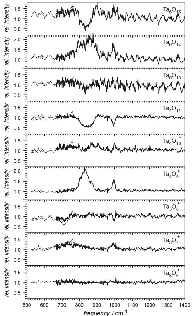
**Fig. 2.** Ion intensity of tantalum oxide cluster cations as function of IR frequency. The spectra are measured in two overlapping frequency scans that are plotted in different styles. Ion intensities are normalized to the signal in the 1100–1400  $\text{cm}^{-1}$  range.
