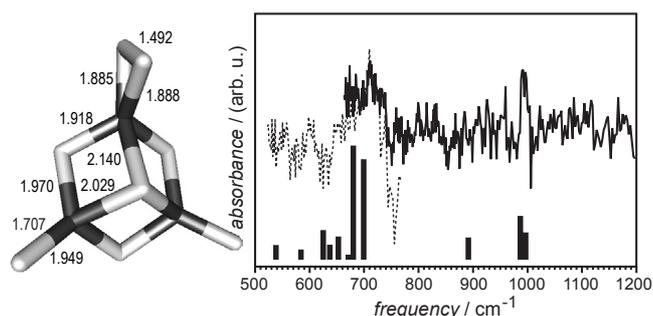
**Fig. 3.** Structure of  $\text{Ta}_3\text{O}_8^+$  ( $C_s$  sym.) and comparison of experimental and calculated IR spectrum. The structure has been optimized with DFT (B3LYP, LACVP\* basis set) using Jaguar 4.0 [22]. The wavenumber axis of the calculated IR spectrum has been linearly scaled to give overlap with the experimental Ta=O stretch frequency resulting in a scaling factor of 0.96.
