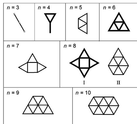
**Figure 3.** Ground-state structures of  $\text{Au}_n^-$  anionic clusters from ref 21 as identified by ion mobility measurements, vertical electron detachment energies, and DFT calculations. These experiments cannot distinguish between two possible structures of  $\text{Au}_8^-$  and both are shown. The structures shown in bold identify the structures deduced from this study.
