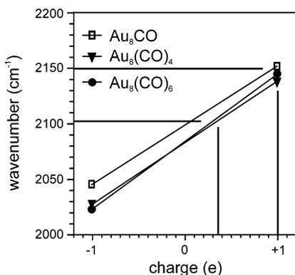
**Figure 5.** Plot relating  $\nu(\text{CO})$  to charge for carbonyls of  $\text{Au}_8$ . Horizontal lines mark the values of  $\nu(\text{CO})$  for CO on deposited  $\text{Au}_8$  particles on defect-rich MgO (lower line) and defect-poor MgO (upper line) taken from ref 4 after conversion from  $\nu(^{13}\text{CO})$  to  $\nu(^{12}\text{CO})$ . The vertical lines mark the corresponding partial charges. It is assumed that the deposited particles are highly covered with CO.
