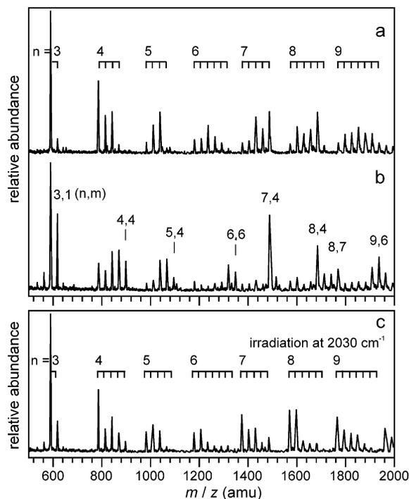
**Figure 1.** Mass spectra of anionic gold cluster carbonyls  $\text{Au}_n(\text{CO})_m^-$ ; the numbers  $(n,m)$  are indicated. The upper trace (a) shows a mass spectrum of gold clusters  $\text{Au}_n^-$ , partially complexed with CO. The middle spectrum (b) is taken at higher  $p(\text{CO})$  where saturation coverage is established. The lower spectrum (c) is obtained when the distribution shown in part b is irradiated at  $2030\text{ cm}^{-1}$ .
