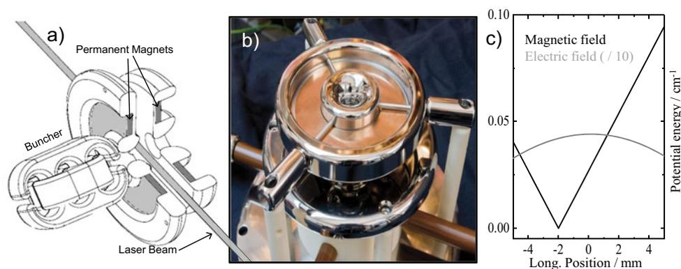
**Fig. 2.** (Color online) Schematic drawing (a) and photograph (b) of the permanent magnetic trap. In (c) the loading potential and the trapping potential for NH ( $a^1\Delta(v=0, J=2)$ ) radicals are shown with respect to the midpoint between the two disc-shaped electrodes.
